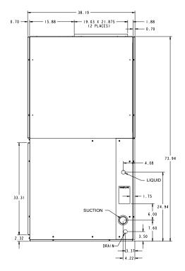
FIGURE 20 - LA300 PIPING CONNECTIONS
